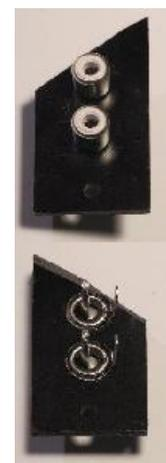
Decide where the plug board will be positioned and drill two holes on the back of the module to accept the two jacks. The centers for these particular plugs are 1/2 inch.
